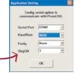
Parani-ESD Series default configuration is 9600 bps Baud rate, 8 Data bits, No. Parity, 1 Stop bit and H/W flow control
