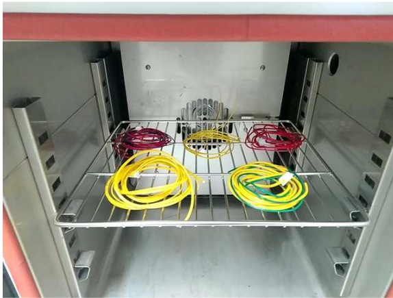
F6-1. sample loading to oven
