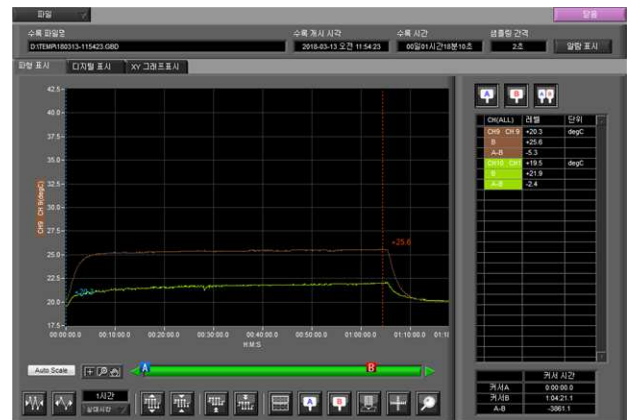
F7-6. Example of test graph (I-21 connector)
